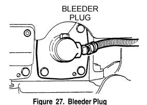
Replace hydraulic oil after first 200 hours and in every 1,000 hours of operation.
